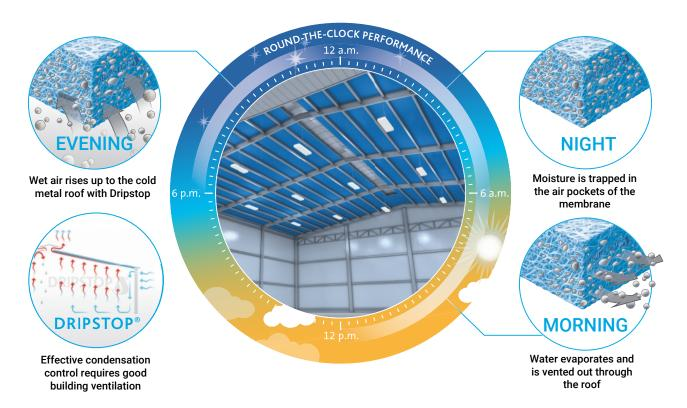
One of the defining poperties of any building is keeping the contents safe from the elements. If condensation from your metal roof is causing your contents to be rained on, your structure is failing in this basic function. Dripstop condensation control is a durable, cost-effective solution to protect your assets.
