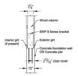
Figure 12.2: Recommended Installation For SWP 8 Series Brackets
